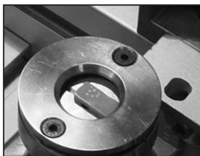
Fig. 2: The test specimen fixed to the wear machine, showing the craters formed.
