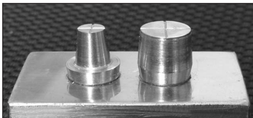
Fig. 2: Lateral view of the metal mold used as a model for taking impressions.
