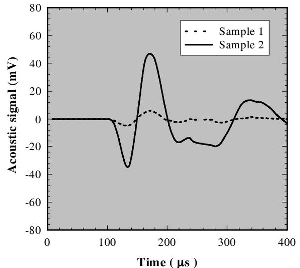
Fig. 2: Amplitude of the acoustic signals detected by the microphone, corresponding to the ablation of two surfaces with different amounts of dirt. The sample 1 is cleaner than the sample 2.
