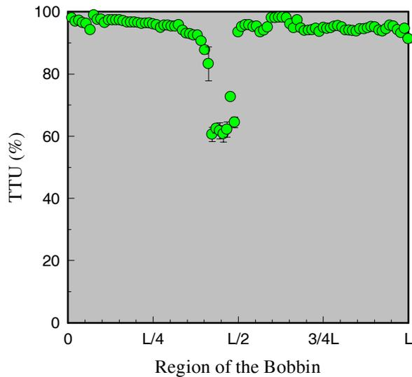
Fig. 8: Measurement corresponding to an oiled coil showing a central region with significant dirt.
