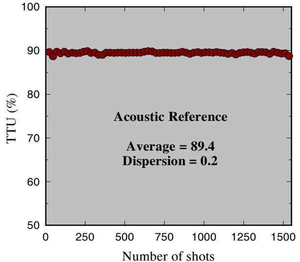
Fig. 6: Measure of the acoustic reference. Each point in the graph corresponds to an average of 24 shots. All the shots impact the same spot of the standard sample, showing that successive shots do not alter the surface.
