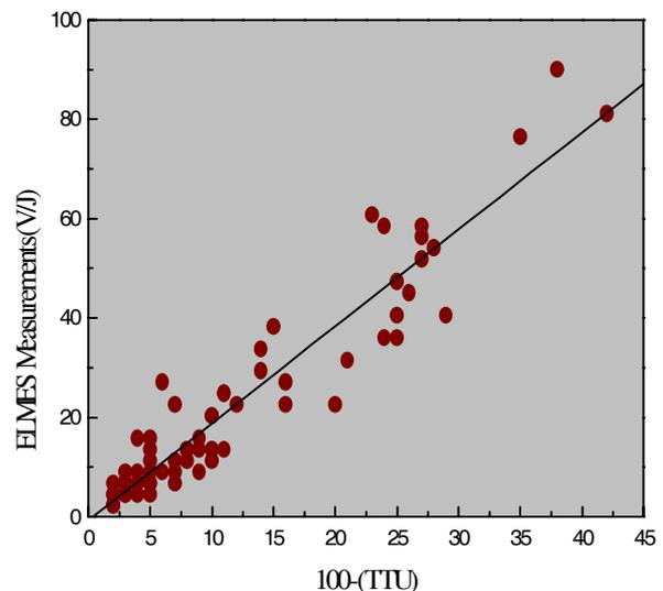
Fig. 3: Correlation between Tape method and ELMES measurements. TTU: Tape Transmission Units.
