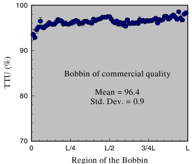
Fig. 7: Measurement obtained with a coil of commercial quality. It indicates that the degree of cleanliness is high and that the residual dirt is homogeneous along all its length.
