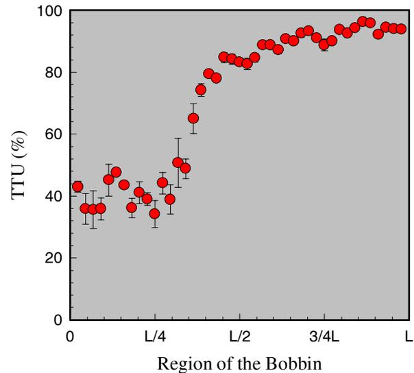
Fig. 9: Measurement corresponding to a coil with two regions of very different cleanliness. Notice that not only the first part is dirtier, but also the dispersion of the dirt is higher.
