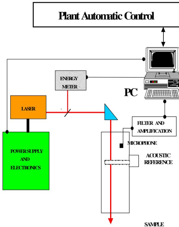
Fig. 1: Schematic of the technique (block diagram of the ELMES).
