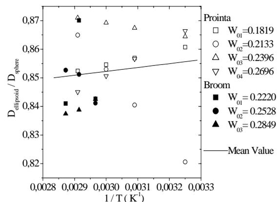
Fig. 4. Ratio of effective diffusion coefficients obtained with ellipsoidal geometry to that found with spherical shape.
