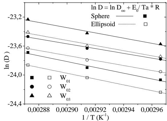
**Fig. 2.** Comparison of Arrhenius-type correlation of cv. Broom diffusion coefficients for sphere and ellipsoid geometry
