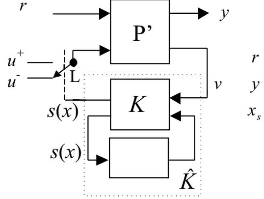
Figure 6: Variable structure system with proposed RM correction
