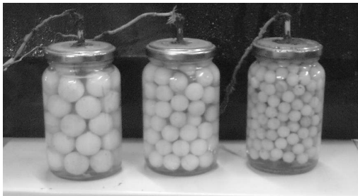
Figure 1: Containers and Samples, Showing the Insertion of Thermocouples through the Lids
