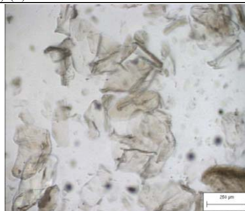
Figure 3. Optical photomicrograph of chitin. The bar represents 250 µm
