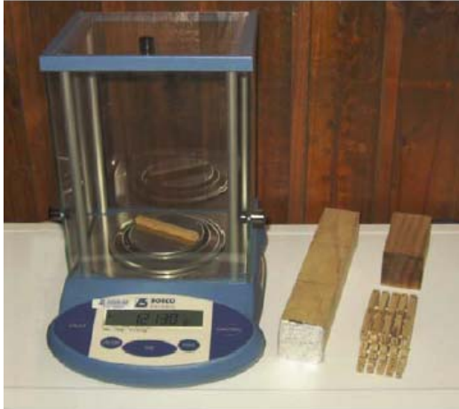
Figure 2. Boeco balance used to determine the mass of each section obtained from blocks P6 and P7.
