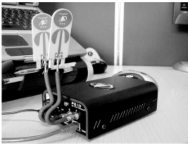
**Fig. 4.** Use of RADAR (RADio Detection And Ranging) techniques. Device developed by our team (reference 28) for telemonitoring in cardiology, with two transmission and reception omnidirectional antennas.
